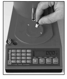
10g weight, and then place the 50g weight on the center of the scale plate. Do not let the weight touch the powder dispense tube.
