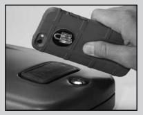
One to five RFID tags can be programmed into the safe.
