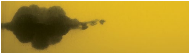
A17 17 HMR (949CC) shot into bare ballistics gel at 100 yards; 6 inches penetration.
