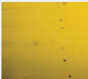
Big 4 38 Special/357 Magnum (3714CC) fired into bare ballistic gel at 10 feet; 6 3/4 inches penetration.
