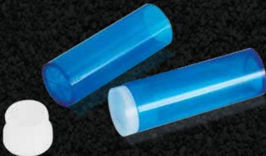
Create custom cartridges with our Empty Shot Capsules. Simply fill them with size 8 or 9 shot (not included), snap in the base wad, and load like a conventional bullet. Shot Capsules include base wads and are available in 44 caliber and 45 Colt (25 count), and 38/357 (50 count). Loading data is available in the Speer Handloading Manual.
