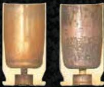
Lawman Clean-Fire spent cases look almost unfired when compared to traditionally primed ammunition. The heavy metals have been removed, producing a clean burn.
