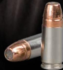
While most self-defense bullets use a deep hollow point to initiate expansion, Gold Dot G2 has a shallow dish filled with an elastomer material. On impact, this material forces the bullet open, providing consistent expansion through any barrier.
