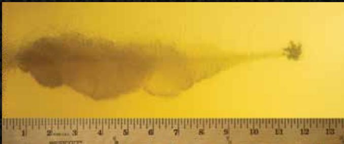
Gold Dot has been proven to provide optimum penetration and expansion through ballistic gelatin and all barriers used in FBI protocol testing. Tests conducted with 9mm Luger 124-grain +P Gold Dot (23617).
