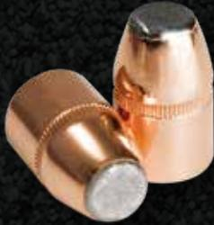
Speer<sup>®</sup> electrochemically bonds the DeepCurl jacket to the lead core to create the toughest, most accurate handgun hunting bullet possible. Pre-formed petals expand reliably and consistently and the bullet's high weight retention ensures deep penetration on heavy-bodied game.
